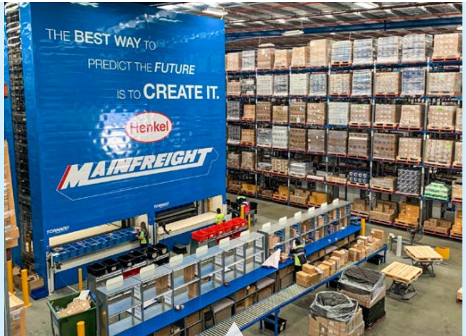
The big blue shiny machine is the VLM and the tote locations opposite to that is the Put Wall
